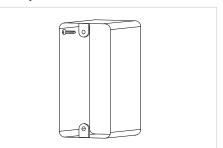
Insert mounting screw into top of junction box until there is approximately 1/8" gap between the screw head and the wall
