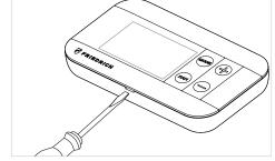
Use a flat head screw driver to separate the front and back housing of the thermostat
