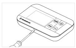
Use a flat head screw driver to separate the front and back housing of the thermostat
